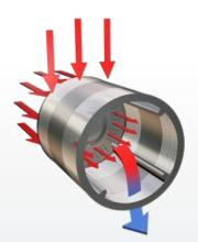
Directing the flow of air through the linen and making the most of their temperature are key factors in getting the best performance from a dryer.
